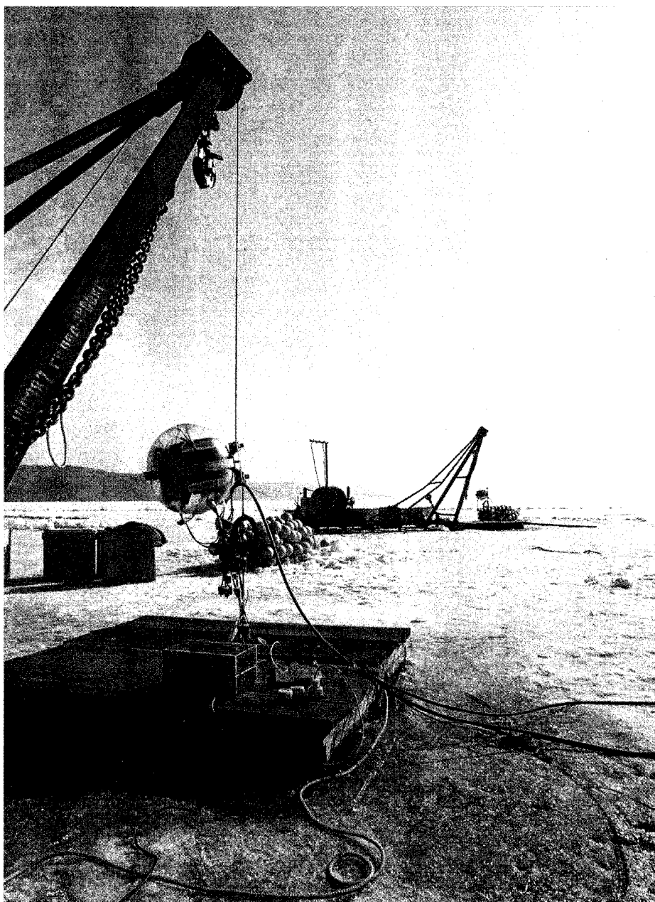
Preparing to immerse components of the Baikal neutrino telescope from the thick winter ice layer. The glass spheres contain 37-cm diameter photomultipliers.
